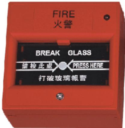
The Call Point can be activated without power supply in emergencies. It is typically located on fire escape doors. The main function is to override the electrical locking devices in case of emergency. Using the provided key to reset the unit to normal mode and to replace the glass.
